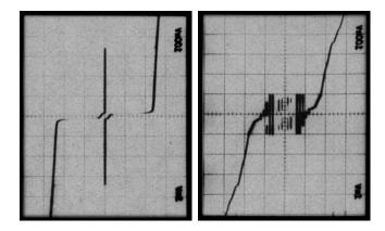
Strongly underdamped superconductor-insulator-superconductor (SIS) junction. The current-voltage characteristic (I horizontal, V vertical) for a Nb–Al<sub>2</sub>O<sub>3</sub> –Nb junction [left] without and [right] with microwave radiation of 70 GHz.
