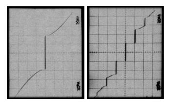
Highly damped superconductor-normal-superconductor (SNS) junction. The current-voltage characteristic (I horizontal, V vertical) for a Nb–PdAu–Nb junction [left] without and [right] with microwave radiation of 10 GHz.
